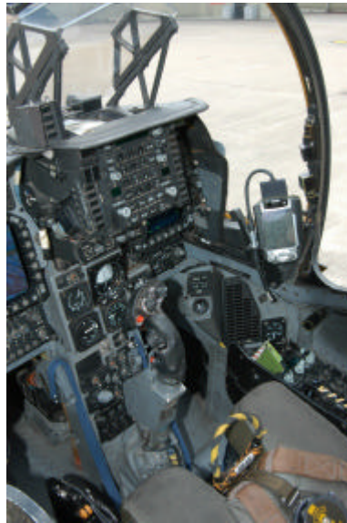
Figure 3: Harrier GR7 Tactical Data Receiver at bottom right of coaming
